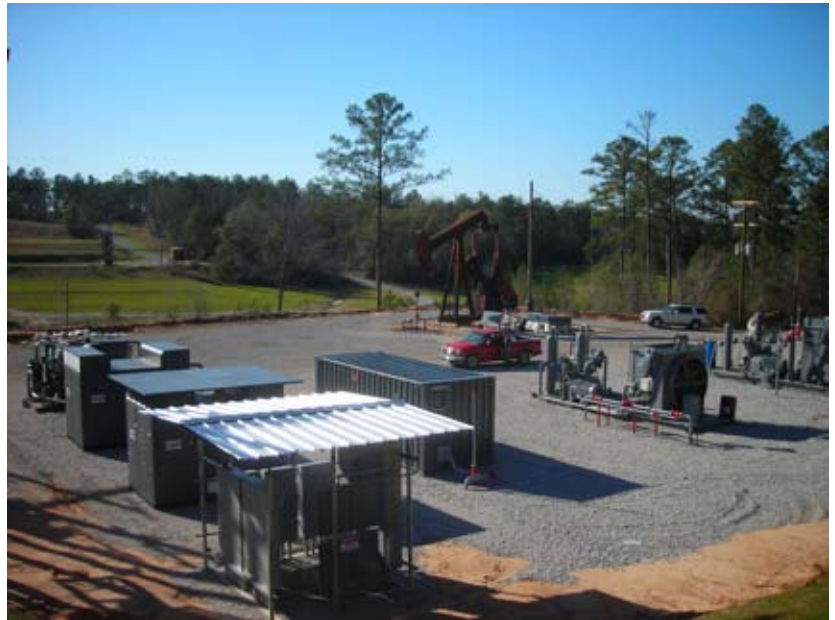
Feed air compressors (left), membrane container (center) and booster compressors (right) on customer's location
